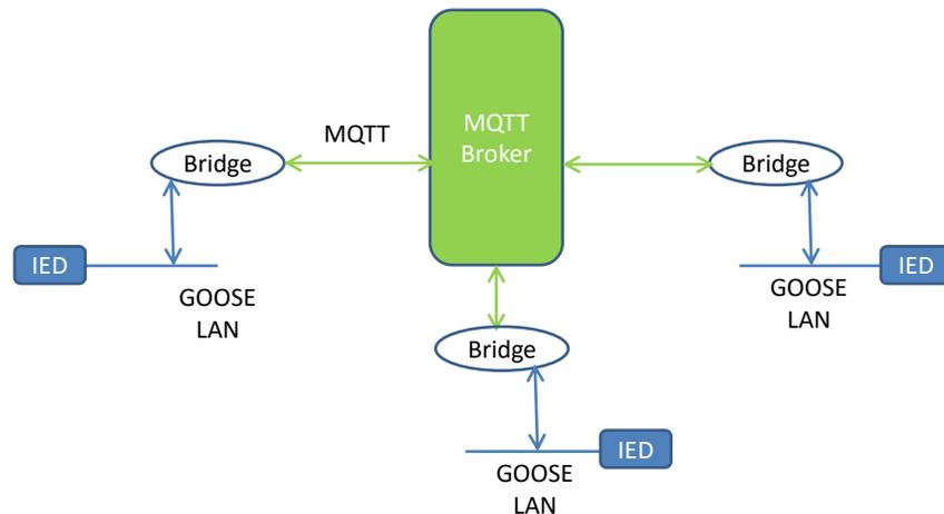
Figure 1: Architecture of GOOSE Exchange using Bridge
