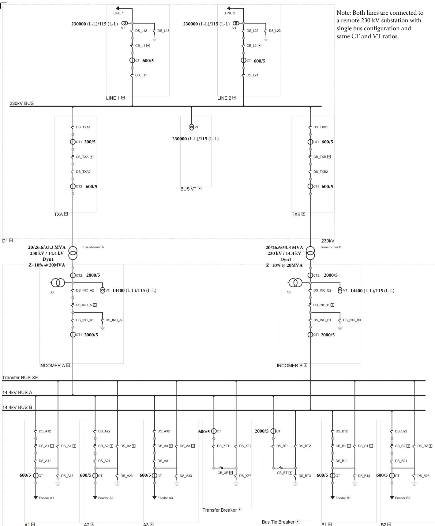
Note: Both lines are connected to a remote 230 kV substation with single bus configuration and same CT and VT ratios.
